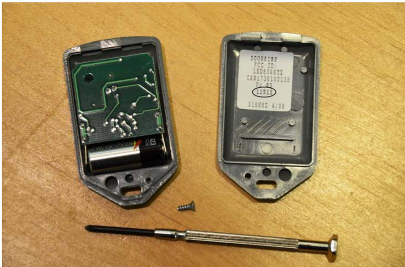
If the label has worn off or is not legible, the old style devices have another label inside the case. You will need to remove the small screw and open the case to find the inside label.
